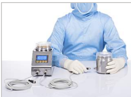
Connection between command unit and satellite
