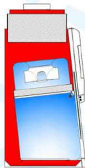
Plenum cast design creates negative pressure around contaminated work area and ensures zero leakage
