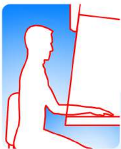
Back sloped front panel design according to anthropometric rules provides increased viewing angle, operator comfort and ergonomic for long period of works
